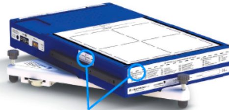
Alignment marks facilitate the TomoTherapy® laser accuracy test (D6)
