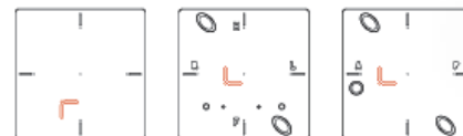
Offset cross-hair markers on the MIMI Phantom, shown in red, are on all sides except the bottom
